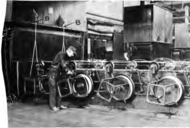
Fig. 1. Automatic Stop for Galvanizing Take-up Frames.*
